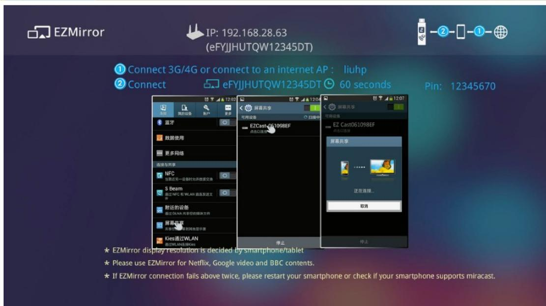
EZMirror is fully compatible with Miracast. You can click the EZMirror button in EZCast app, and the receiver will be switched to Miracast mode.
