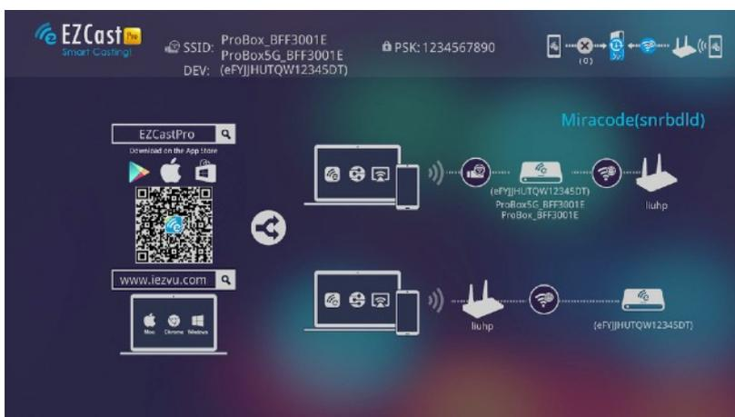
Via Router Allowed: You will be able to discover EZCast Pro through home router if you have established the connection with router.
